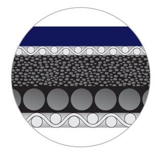
COLOUR Indigo FACE COMPOUND For UV and oxidation ink drying systems CONSTRUCTION **Cord Carcass** TYPE Compressible SURFACE FINISH Ground and polished SURFACE ROUGHNESS, RA  $0,60 - 0,90 \, \mu m$ 68 +/- 3 IRHD MICRO HARDNESS < 0,70 % at 500 N/5 cm STRETCH NOMINAL THICKNESS 1,95 mm (ISO 12636) 1,69 mm (ISO 12636) GAUGE LOSS ≤ 0,02 mm
